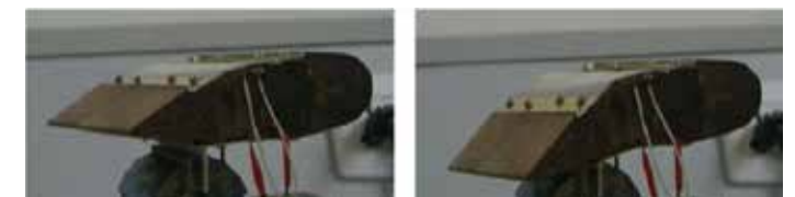
Variable-camber wing based on shape memory polymer skin
